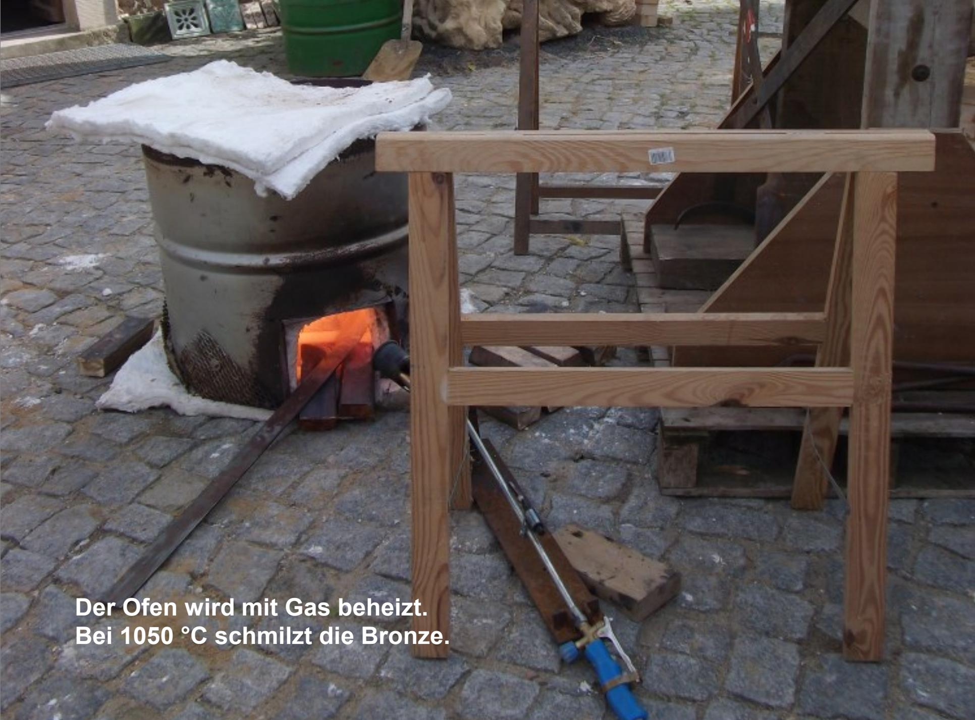
A gas furnace, constructed from a metal barrel, sits on a cobblestone floor. A bright orange flame is visible from a gas burner at the base of the furnace. A wooden frame, made of light-colored wood, is positioned in front of the furnace. A gas torch with a blue handle and a silver nozzle lies on the ground in the foreground. In the background, there is a green barrel, some wooden blocks, and a wooden structure.
